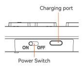
2. Switch the keyboard power to the ON position.
