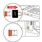
1. Plug the USB receiver into a USB port on your computer.
