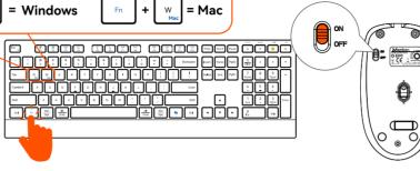
4. Press FN+O to switch to the Windows system, and press FN+W to switch to the Mac system. All indicators will blink three times, when the switching is successful.
