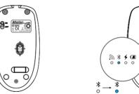
2. Click the 'Mode Switching Button' to switch to Bluetooth mode. The corresponding Bluetooth indicator will light up blue and start blinking.
