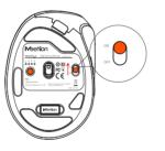
1. Togale the switch upward to the "ON" position to turn the device on.
