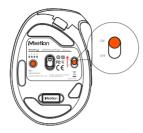
4. Toggle the switch upward to the "ON" position to turn the device on.
