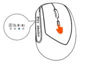
2. Click the "Mode Switching Button" to switch to Bluetooth 1 / Bluetooth 2 mode, the corresponding Bluetooth 1 / Bluetooth 2 indicator will light up blue and start blinking.
