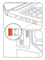
1. Insert the USB receiver into the USB port of your computer.
