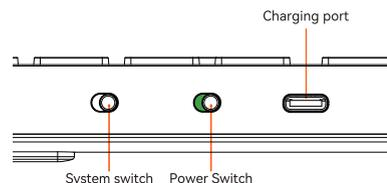
1. Press the button to move to the right to open the device.
