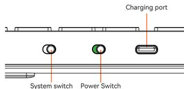
2. Press the button to move to the right to open the device.
