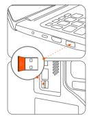
1 Insert the USB receiver into the USB port of the computer.
