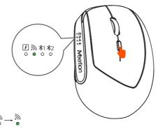
2. Click the "Mode Switching Button" to switch to 2.4G mode,the corresponding 2.4G indicator will light up green.
