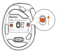
1. Toggle the switch upward to the "ON" position to turn the device on.
