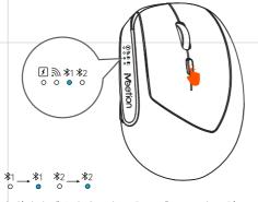
2. Click the "Mode Switching Button" to switch to Bluetooth 1/2 mode, the corresponding Bluetooth 1/2 indicator will light up blue and start blinking.
