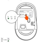
**5.** Click the 'Mode Switching Button' to switch to 2.4G mode. The corresponding 2.4G indicator will light up green. Get ready!
