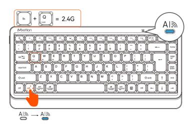
**3.** Press the "FN" key and then the "Q" key to switch to the 2.4G mode. The indicator light will turn on.
