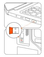
**1.** Plug the USB receiver into a USB port on your computer.
