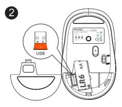
Pull out the USB receiver on the bottom of the mouse
