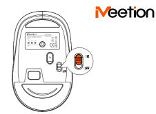
**4.** Toggle the switch upward to the 'ON' position to power on the device.
