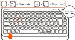
2. Press the "FN" key + "W" key to switch to Bluetooth 1 mode, Press the "FN" key + "E" key to switch to Bluetooth 2. At this time, the corresponding indicator lights will illuminate.
