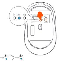
2. Click the "Mode Switching Button" to switch to Bluetooth mode, the corresponding Bluetooth indicator will light up blue and start blinking.
