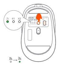
3. Click the "Mode Switching Button" to switch to 2.4G mode, the corresponding 2.4G indicator will light up green, get ready!
