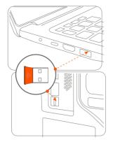
1. Insert the USB receiver into the USB port of your computer.
