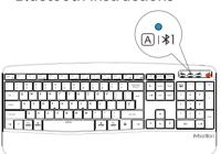
1. Click \$1 / \$2 button to switch to Bluetooth / Bluetooth 2 mode, the corresponding Bluetooth 1 / Bluetooth 2 indicator will light up blue and start blinking.
